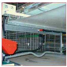
The secondary scraper placed on the return side of the manure belt before the last cage stand in an area undisturbed by feathers grants maximum cleaning.
