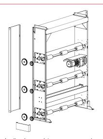
In the heavy duty manure removing unit steel sprockets ensures maximum durability and are designed to facilitate inspection and maintenance.
