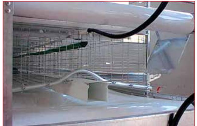
The solution with manure drying duct under the cage is ideal for moderate length sheds and allows to utilize the full cage depth. The special design with the duct all over the floor wire mesh grants a complete cleaning of the manure duct upper part done by the birds' feet.
