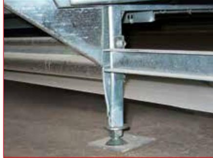
The special shape of the lower part of the cage stand ensures greater static stability while the adjustable cage base element allows to compensate unevenness of the shed's floor for perfect leveling.
