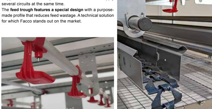
FACCO drop-type nipple drinkers are effective and precise. They ensure that an adequate and waste-free supply of water is dispensed with optimum performance for all the birds. The Facco nipple drinkers are positioned exclusively at nest level, at the front and respectful of animal welfare throughout the daily life and egg-laying cycle of the birds.
