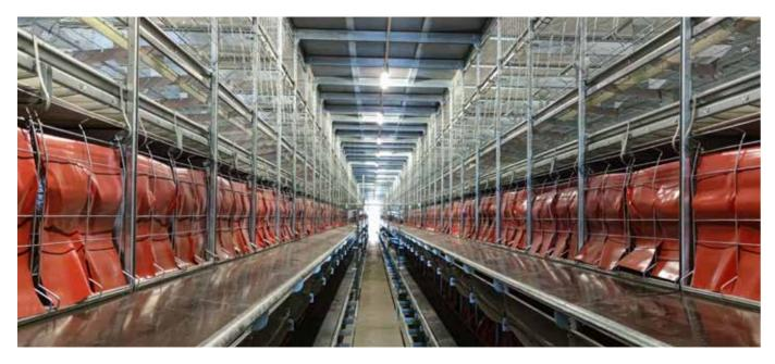
The slightly sloping base of the nest and treading surface allows the eggs to gently slide towards the egg collection belt, which is made of perforated polypropylene, a material that is very easy to clean. When it comes to egg collection, the lateral position of the nest, towards the aisle, facilitates:
