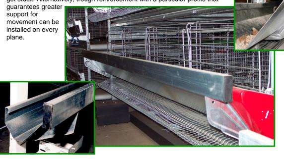
As an optional, the system can be provided with an egg-saving system that enables reducing the breakage rate due to collision, automatically releasing the eggs at regular intervals.
